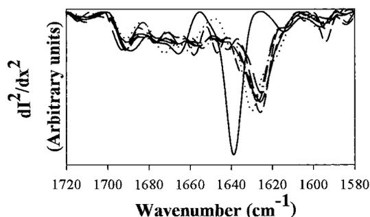
FIG. 3. Second-derivative amide I FT-IR spectra for native SMA (solid line), pure SMA amyloid fibrils (dotted line), and pressure-induced aggregates generated at 80 (long dashed line), 120 (medium dashed line), 160 (short dashed line), 200 (dashed-dotted line), and 240 (dashed-dotted-dotted line) MPa.
