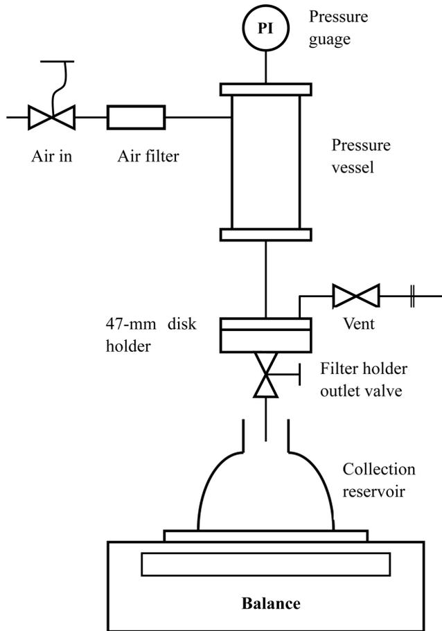
**Fig. 2.** Filtration apparatus for process optimization and virus validation study using a Viresolve NFP disk membrane. The filtrate volume was recorded by measuring the filtrate mass using a balance.
