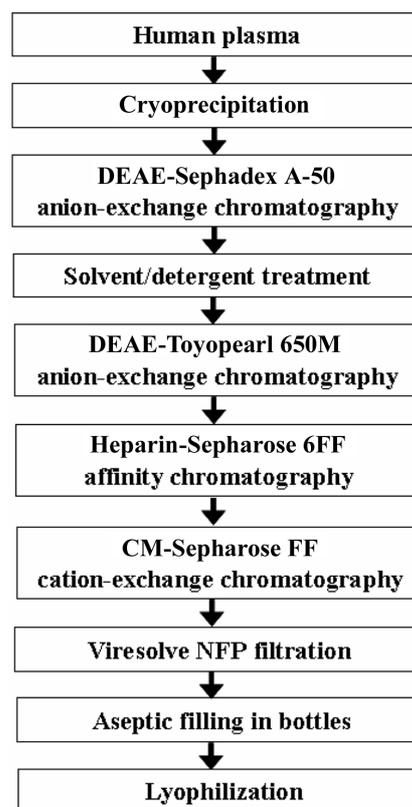
**Fig. 1.** Flow diagram of the manufacturing process for high-purity factor IX from human plasma.
