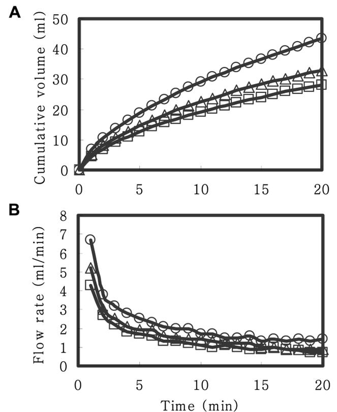
**Fig. 5.** Effect of operating temperature on the cumulative filtration volume (A) and flow rate (B) of factor IX solution through Viresolve NFP disk membrane.
