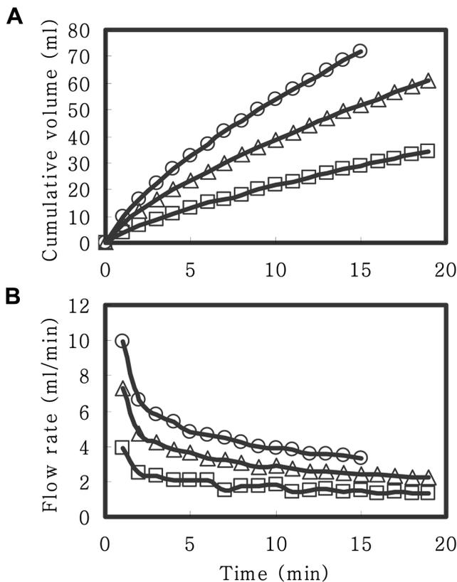
**Fig. 4.** Effect of operating pressure on the cumulative filtration volume (A) and flow rate (B) of factor IX solution through Viresolve NFP disk membrane.
