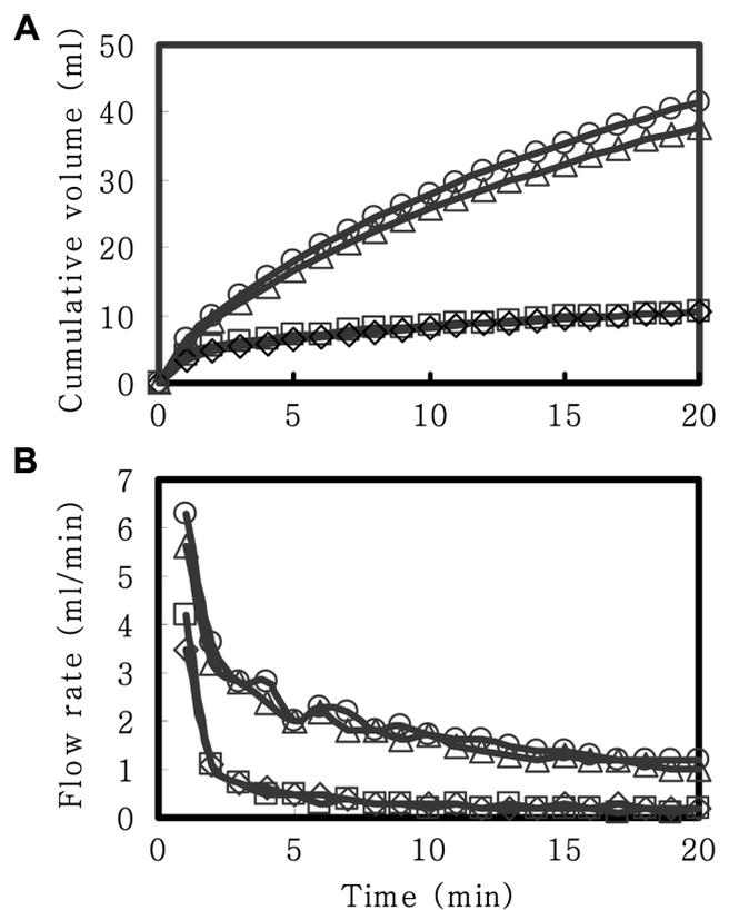
**Fig. 3.** Effect of operating pH on the cumulative filtration volume (A) and flow rate (B) of factor IX solution through Viresolve NFP disk membrane.
